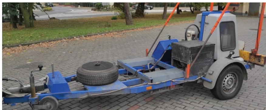
Fig. 1. Dynatest® – falling weight deflectometer
