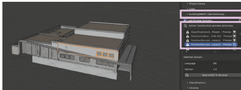
Fig. 1. Loading the bSDD dictionary into the Blender application with the usage of the Bonsai plug-in
