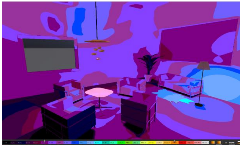
Fig. 4. Visualisation of luminance distribution in an apartment depicted with false colours, made with DIALux evo software
