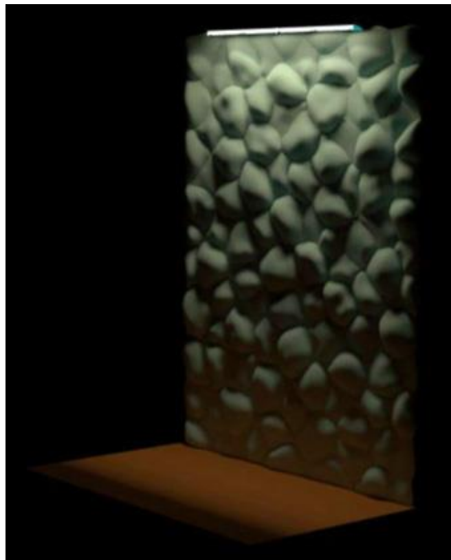
Fig. 6. An example of the proper visualisation of the light distribution on a structural wall. The visualisation was made using Photopia software in the Rhino environment
