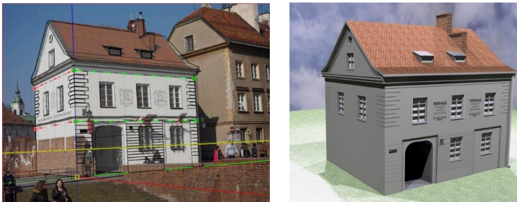
Fig. 2. Illustration of the process of creating a three-dimensional model of a tenement house from a photo. The tenement house is located in the Old Town of Warsaw. SketchUp software was used to create the building model, while the digital model was made using a hand modelling technique
