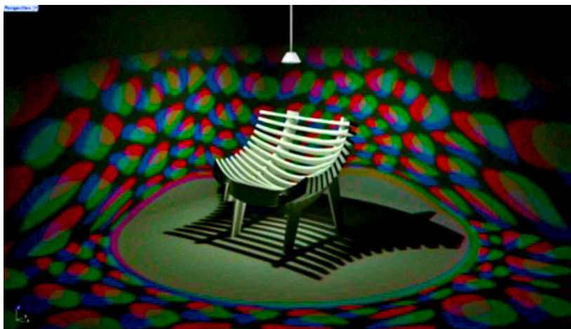
Fig. 5. Visualisation of light distribution considering the spectral distribution of light sources in a room illuminated with a luminaire with blue, red and green LEDs
