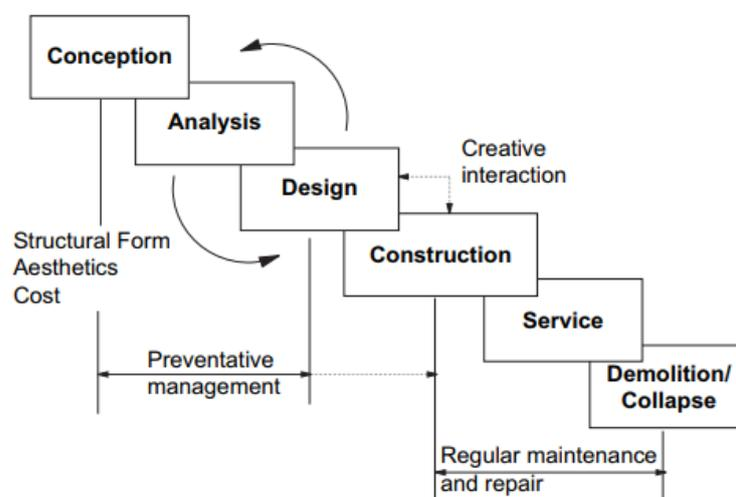
**Fig. 1.** Stages of the bridge life cycle
