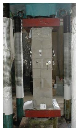
**Fig. 2.** General view of the testing of a specimen column
