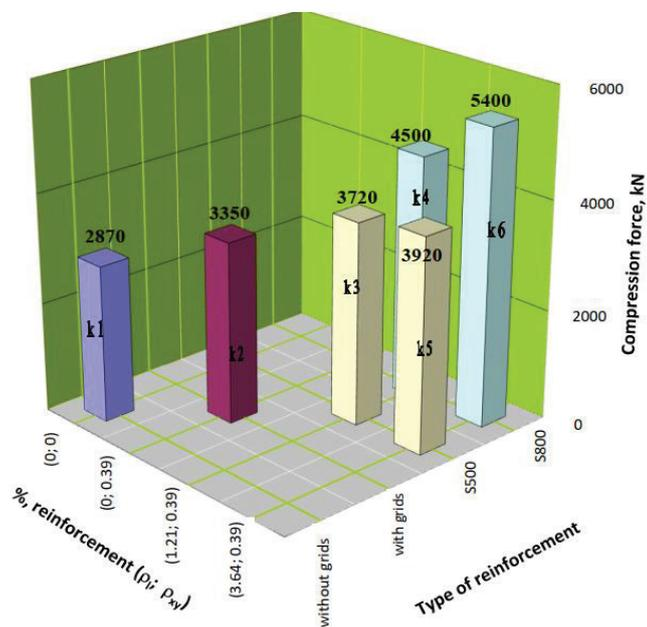
**Fig. 5.** Strength of specimens with different reinforcement
