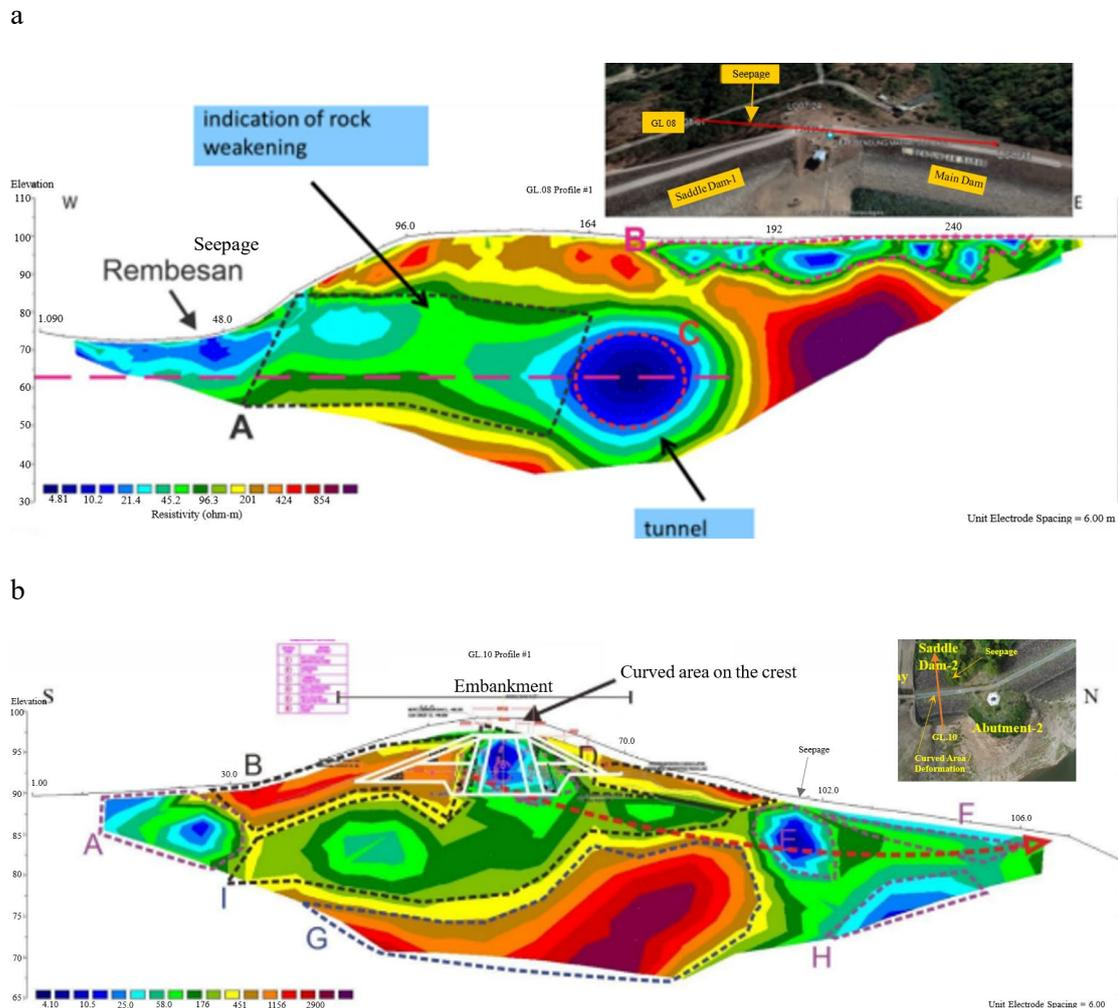
**Fig. 3.** Goelectric investigation: a – Goelectric survey Line 8 (GL8) in Saddle Dam-1, b – goelectric survey Line 10 (GL10) in Saddle Dam-2
