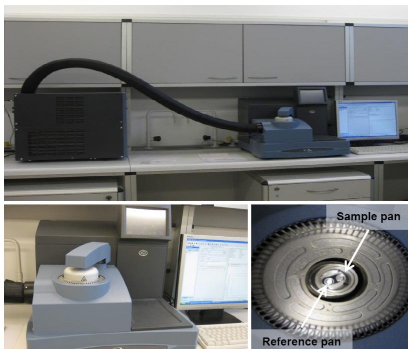
Fig. 3. Differential Scanning Calorimeter Q200 oxidation induction time apparatus
